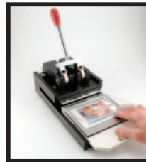
1. Align photo in desired die.
