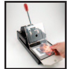
4. Release handle, pull out die and remove photo.
