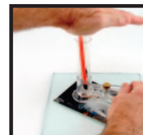
Place one palm on top of center tube with the other hand on blade arm. With downward pressure turn blade arm one full clockwise turn.
